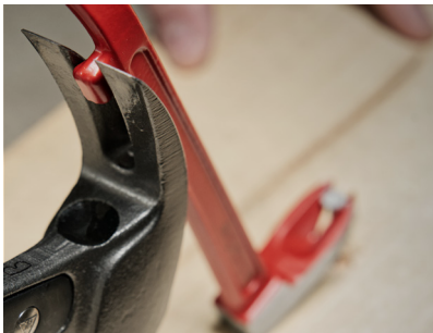
The claw hammer interaction provides extra leverage for larger nails.
